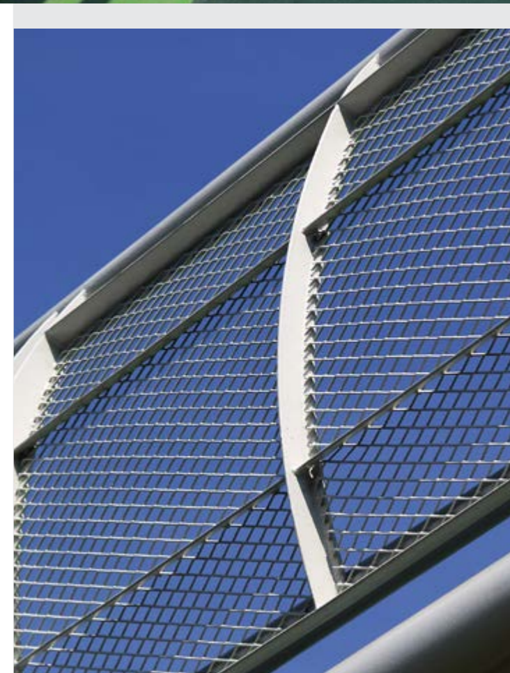
Material used: Railing filling Type: expanded metal / diamond mesh MR 90 x 31,5 x 4 x 3 mm Material: hot dipped galvanized steel + painted
